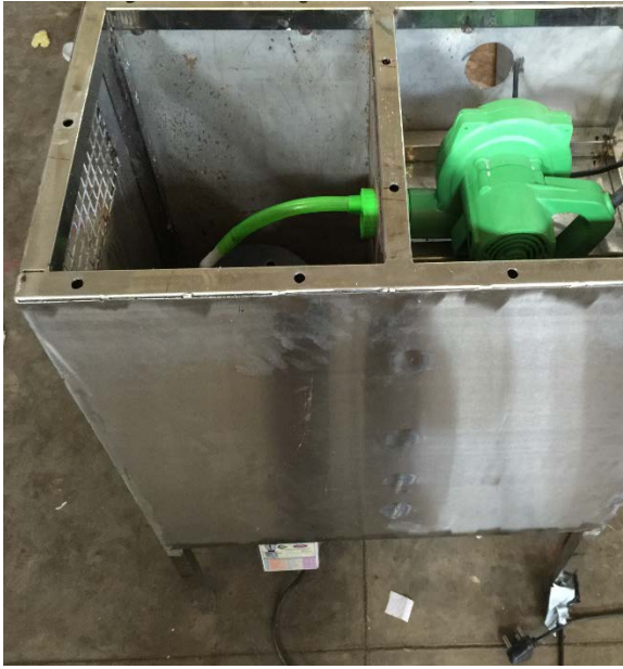
Fig8 Arrangement of blower in halogenerator.
